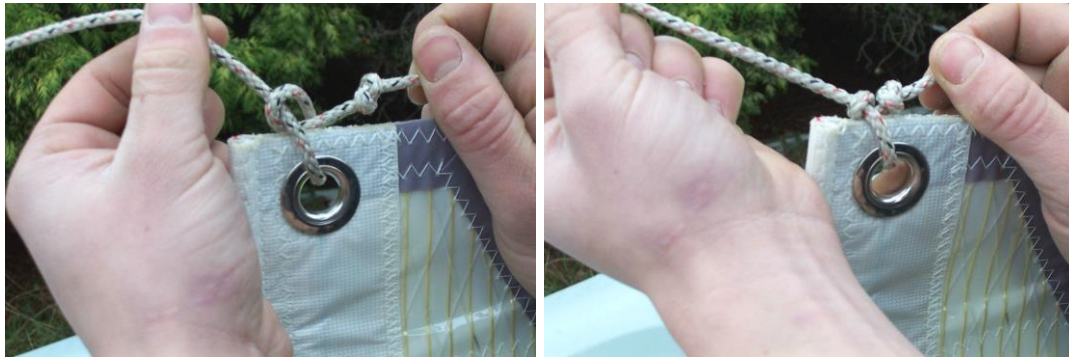
Picture 3.27 Tying the Main Halyard
