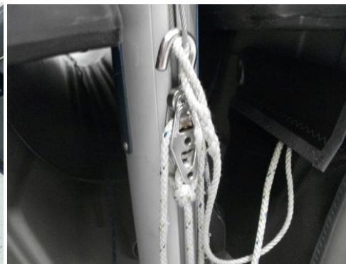
Picture 3.20 Connecting the Rig Tension
