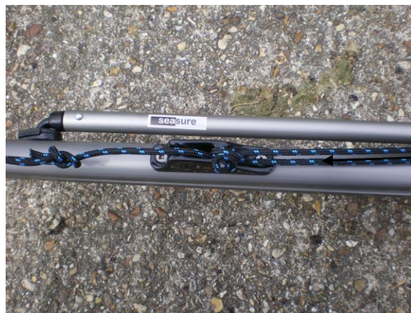
Picture 3.23 The Rudder Downhaul
