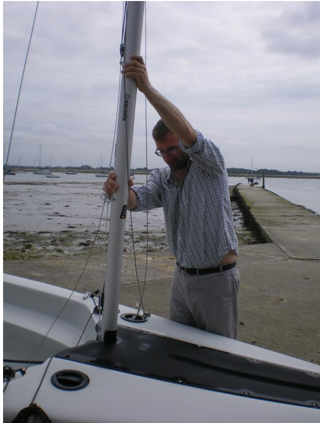
Picture 3.5 Stepping the Mast Single Handed
