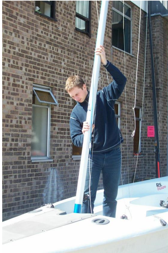
Picture 3.8 Stepping the Mast
