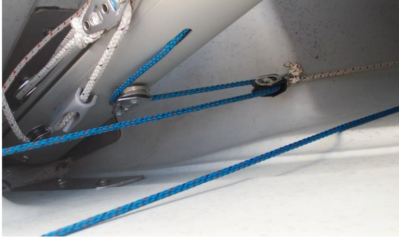
Picture 3.10 Threading the Gennaker Halyard
