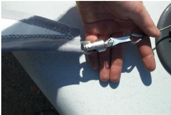
Picture 3.19 The Head of the Jib Attached
