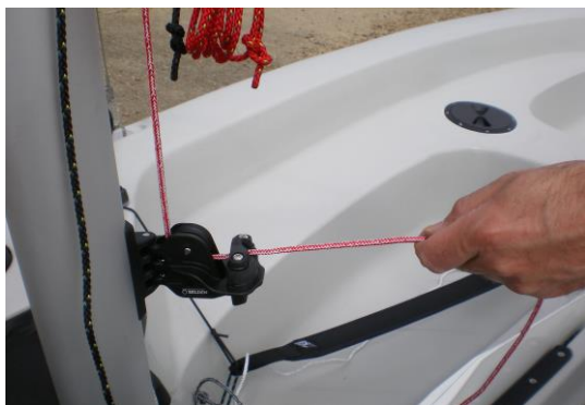
Picture 3.15 The Gnav Control Line
