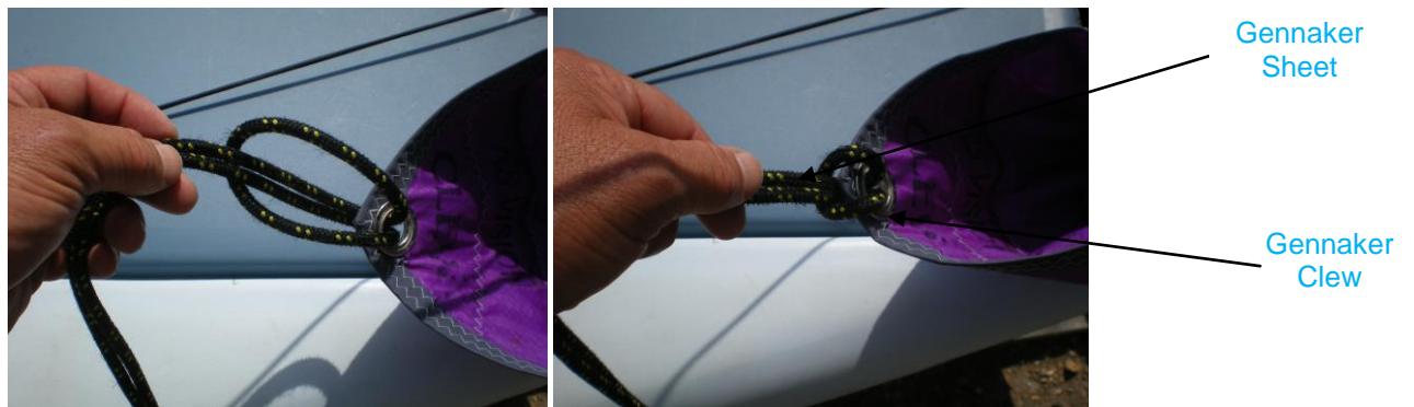
Picture 3.35 Attaching the Gennaker Sheet
