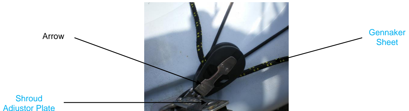
Picture 3.36 The Gennaker Sheet Block
