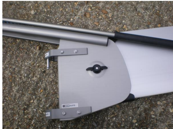
Picture 3.22 The Rudder Fitted in the Stock
