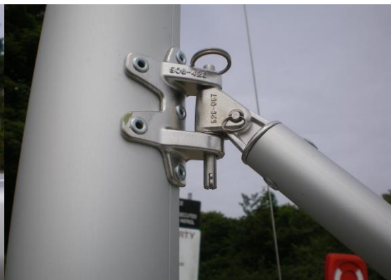
Picture 3.14 Connecting the Gnav to the Mast
