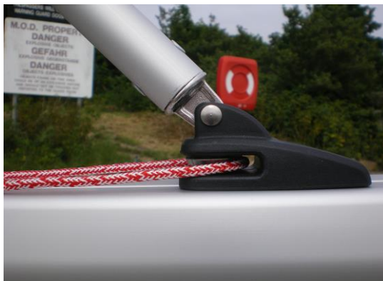
Picture 3.13 Connecting the Gnav to the Boom
