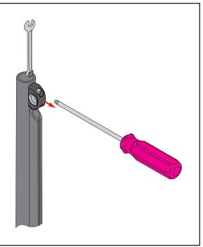
3) Insert the Backing plate (AER-SP-916) into the mast and line up with existing holes, hold this in place with a finger while lining up the bullseye holes.
