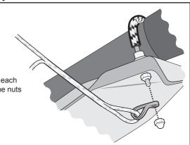
Add the P-clips onto the bolts on each side of the boat. Replace the dome nuts and tighten.
