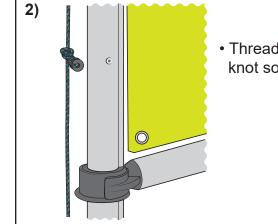
• Thread the halyard through the sheave and tie a double overhand knot so sheave is level with rivet as shown in picture.
