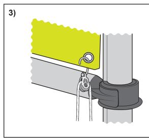
• Take the top block (with hook) and connect to the downhaul cringle at the tack of the mainsail.
