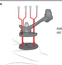
Add the new mainsheet swivel base on top of the old base using the 4 machine screws provided.
