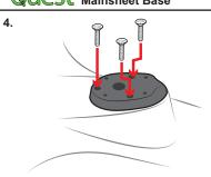
Screw the base back onto the boat using the screws removed in step 2.
