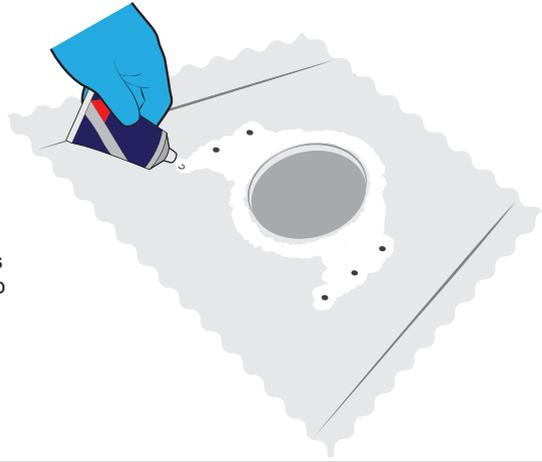
Use Sikaflex to seal the screws and to bed the collar down onto the deck.
