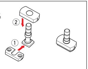
Push the Universal Joint assembly into the end of the tiller extension, make sure it is completely inserted.
