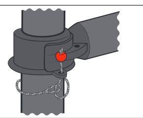
Cut off any excess tail and seal the end.
