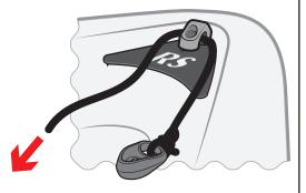
c) Take the end aft and pass it underneath the organiser on the starboard side of the mast step.
