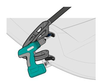
4. Use the M6 x 30, Penny washer and Nyloc. Dont forget the Sikaflex sealant. Tighten the fitting
