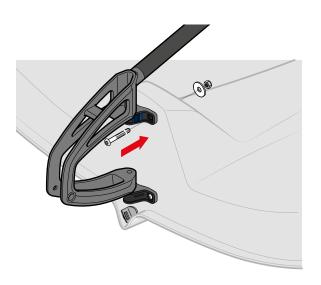
5. Repeat for the other screws in the numbered order one fixing at a time
