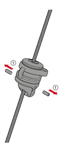
1. Remove large grub screws from side of swivel
