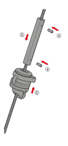
4. fit the long plastic insert and insert the grub screws
